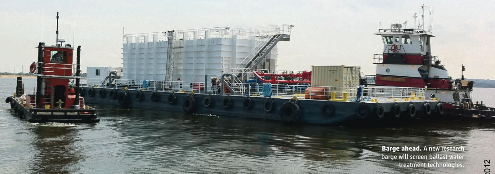
**Barge ahead.** A new research barge will screen ballast water treatment technologies.
